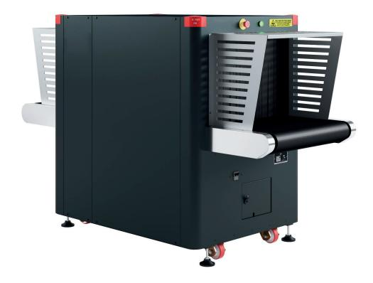
Professional multi-energy X-ray system for the control of packages and parcels and baggage of medium-small size in general; allows the identification of organic and inorganic materials, including explosives and drugs and the identification of weapons, trigger devices and dangerous objects that can create security risks.
